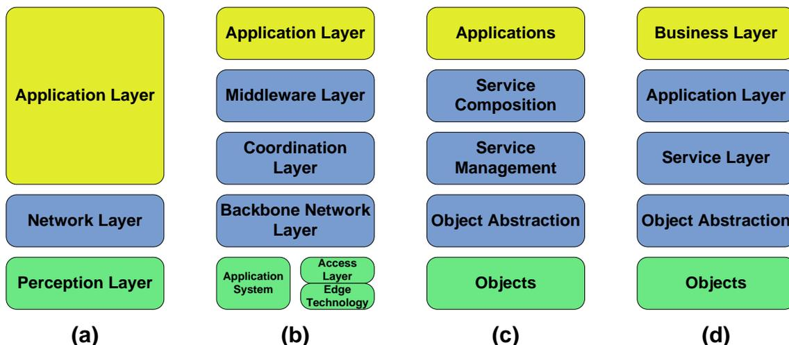
Figure 4: Comparison of proposed IoT architectures (a) Three-layer, (b) Middleware based, (c) SOA based, (d) Five-layer
